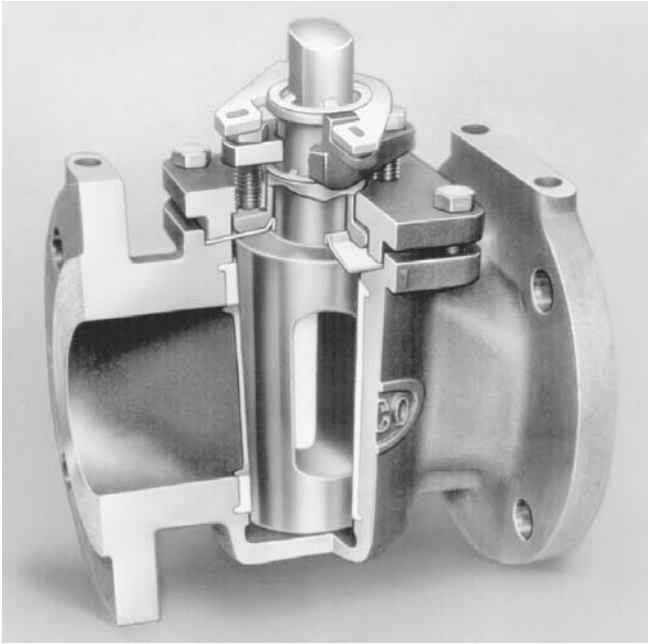
Figure 3.1 Nonlubricated, PTFE-sleeved quarter-turn plug valve. (Courtesy of The Duriron Company, Valve Division)
