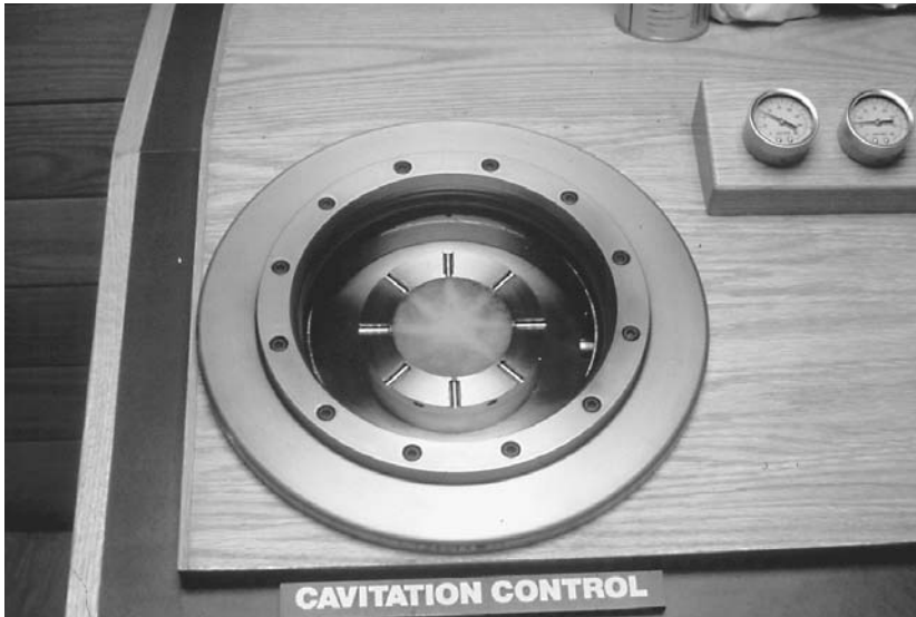
Figure 9.11 Laboratory experiment showing diversion of cavitation away from boundary surfaces using cavitation control trim. (Courtesy of Valtek International)
