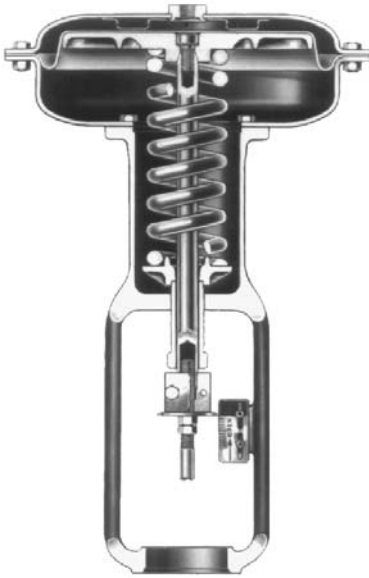
Figure 5.9. Direct-acting diaphragm actuator. (Courtesy of Fisher Controls International, Inc.)
