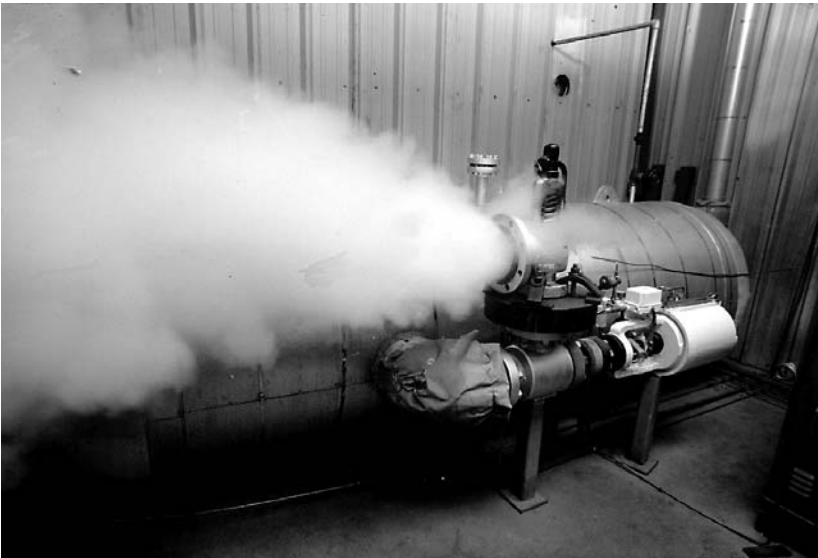
Figure 1.4 Pressure-relief valve being tested for correct cracking pressure. (Courtesy of Valtek Houston Service Center)
