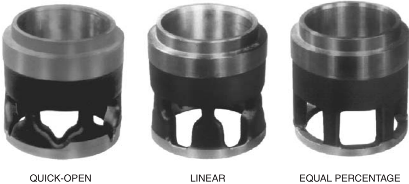
Figure 2.2 Characterizable cages. (Courtesy of Fisher Controls International, Inc.)
