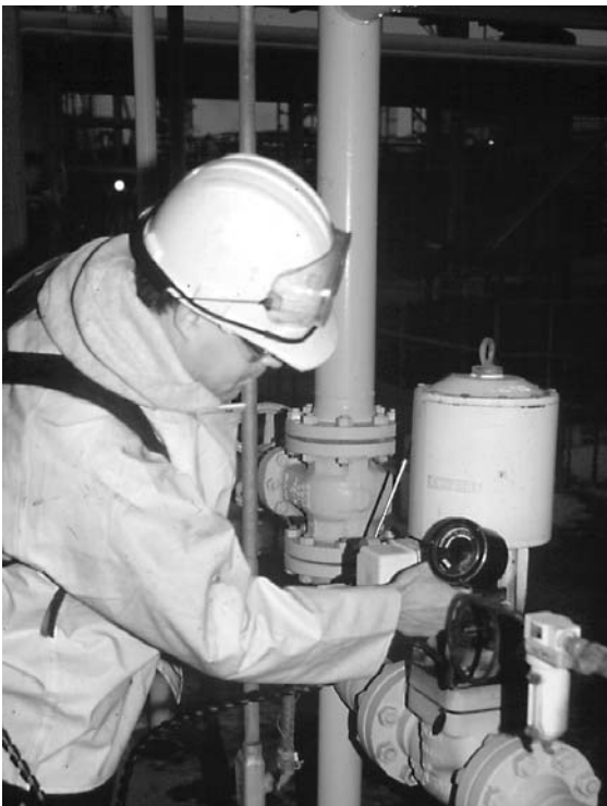
Figure 9.56 Organic sniffer used to detect fugitive emissions. (Courtesy of Valtek International)
