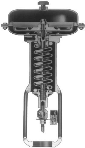
Figure 5.10. Reverse-acting diaphragm actuator. (Courtesy of Fisher Controls International, Inc.)
