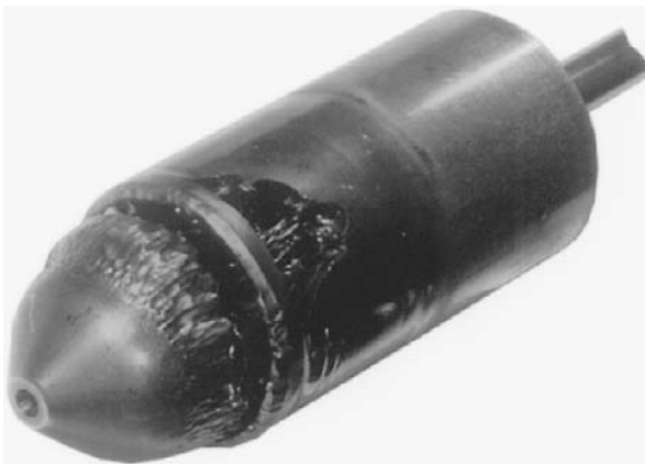
Figure 9.23 Plug damaged by flashing. (Courtesy of Fisher Controls International, Inc.)
